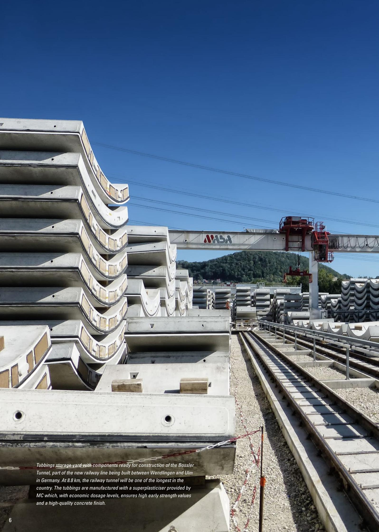
*Tubbing storage yard with components ready for construction of the Bossler Tunnel, part of the new railway line being built between Wendlingen and Ulm in Germany. At 8.8 km, the railway tunnel will be one of the longest in the country. The tubbing are manufactured with a superplasticiser provided by MC which, with economic dosage levels, ensures high early strength values and a high-quality concrete finish.*
