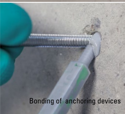
Bonding of pull-off heads
