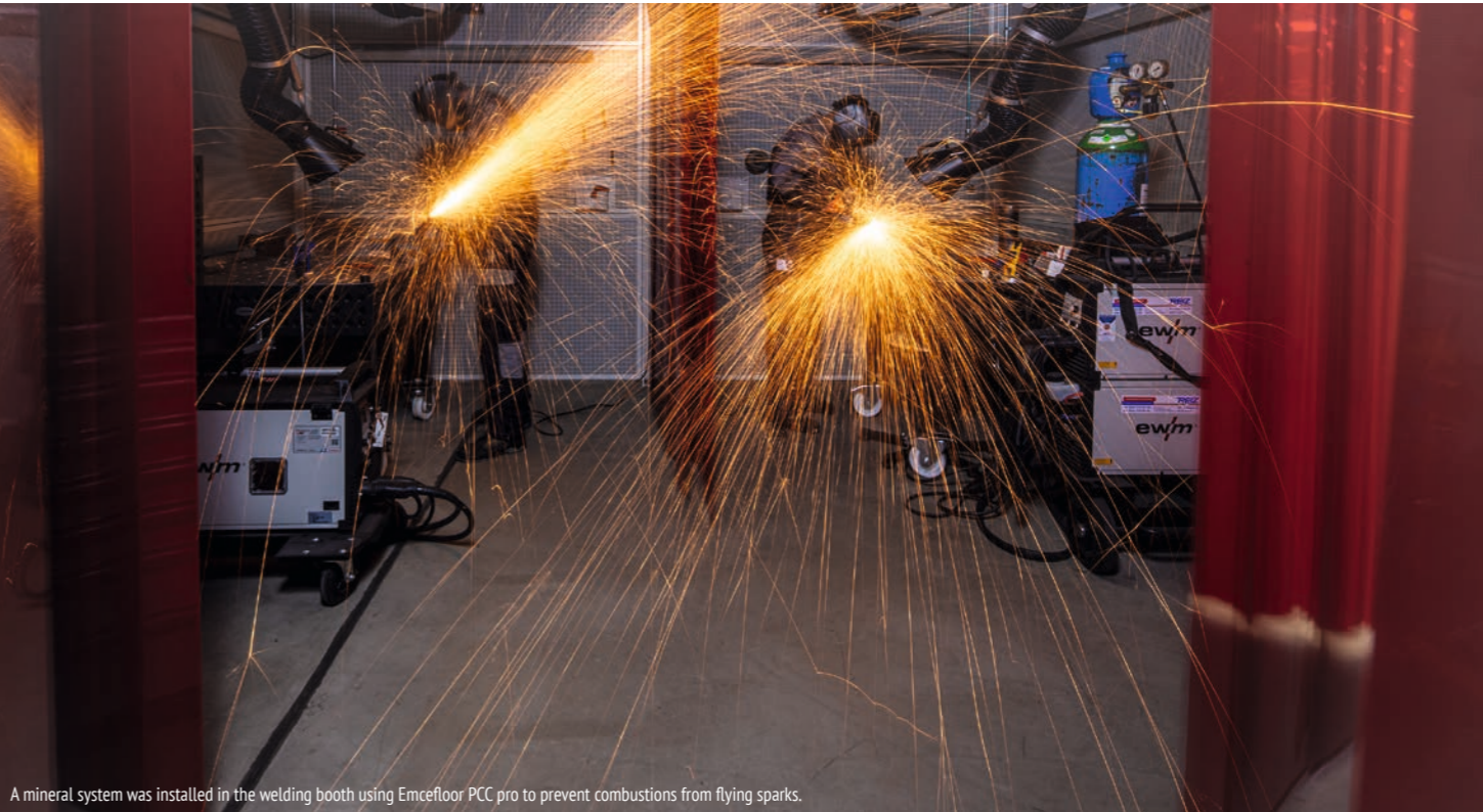
A mineral system was installed in the welding booth using Emcefloor PCC pro to prevent combustions from flying sparks.
